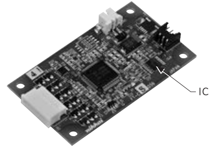
Change of IC Chip for FT Series Controller Board
