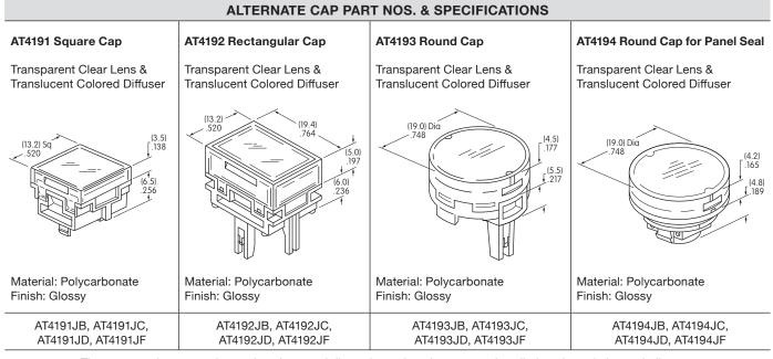
There are no changes to the products' external dimensions when the caps are installed on the switches or indicators. Contact information is below if more details are needed.
