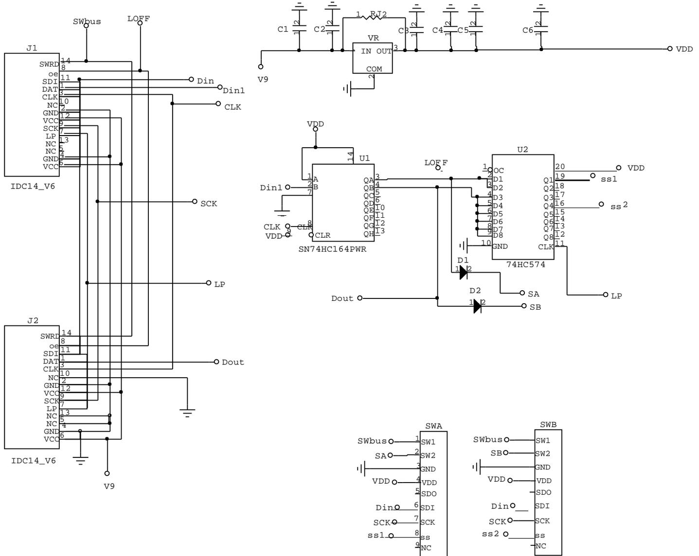
**IS-L06A1, logic board, six 64x32 RGB Pushbuttons**
