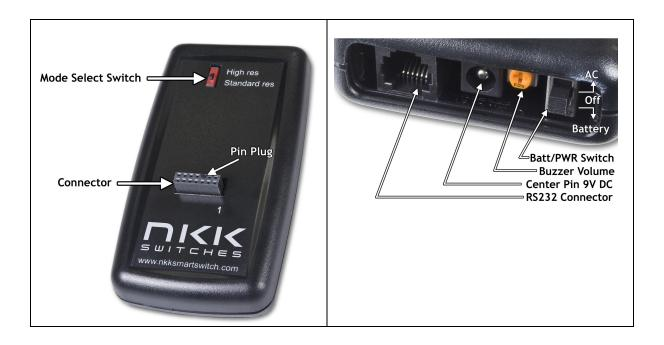
The **Mode Select Switch** has two settings; "High res" is for the LCD 64x32 (64x32) switches/ displays and "Standard res" is for the LCD 36x24 RGB switches/ displays.
