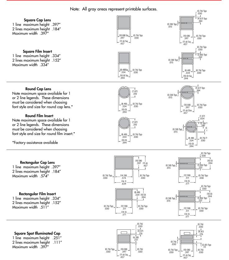
Note maximum space available for 1 or 2 line legends. These dimensions must be considered when choosing font style and size for round printable area of cap lens or film insert.
