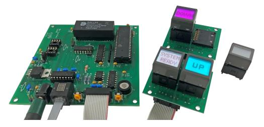
The purpose of the Modular HMI System is to allow flexibility of placement of switches on control panels. The system is made up of a controller and several SmartDisplay populated PCBs connected by ribbon cables.
