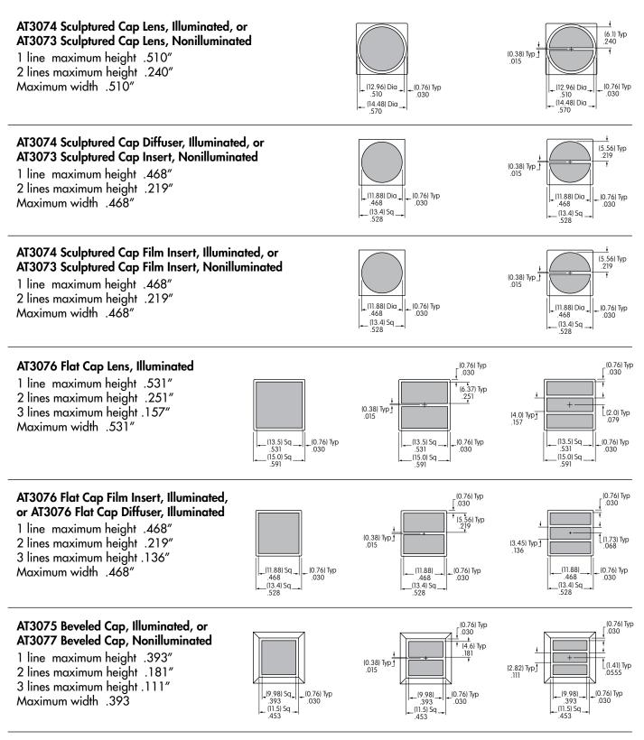
For Sculptured: Note maximum space available for 1 or 2 line legends. These dimensions must be considered when choosing font style and size for round printable area of cap lens, diffuser, insert or film insert.
