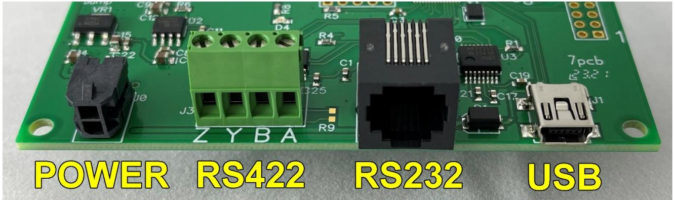
**Power Connector:** Molex 0430450200, top position power, bottom position ground.
