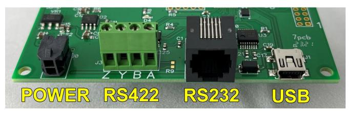
**Power Connector**: Molex 0430450200, top position power, bottom position ground. Mating: Molex 0430250208
