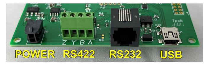
**Power Connector**: Molex 0430450200, top position power, bottom position ground.
